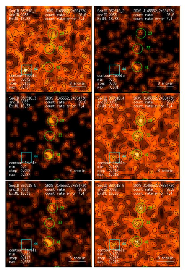
Figure 33: RASS 930518: detection 0033: band rate images, Gaussian filter: (1) PSPC channels 11 - 41, (2) 52 - 90, (3) 91 - 201, (4) 11 - 235, (5) 52 - 201, (6) 11 - 201. Broad band rates in counts/ks. Band rate contour levels in counts/ks/arcmin<sup>2</sup>.
