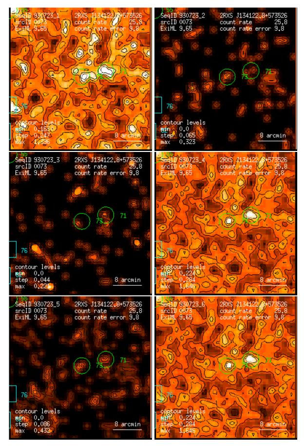
Figure 73: RASS 930723: detection 0073: band rate images, Gaussian filter: (1) PSPC channels 11-41, (2) 52-90, (3) 91-201, (4) 11-235, (5) 52-201, (6) 11-201. Broad band rates in counts/ks. Band rate contour levels in counts/ks/arcmin<sup>2</sup>.
